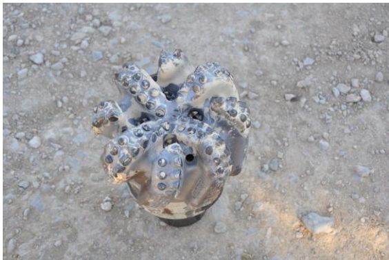
Figure 7. Bit 1 after removal at 2070 ft.
