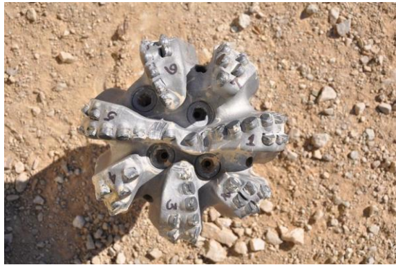
Figure 11. Bit 2 after being pulled at 2634 ft.
